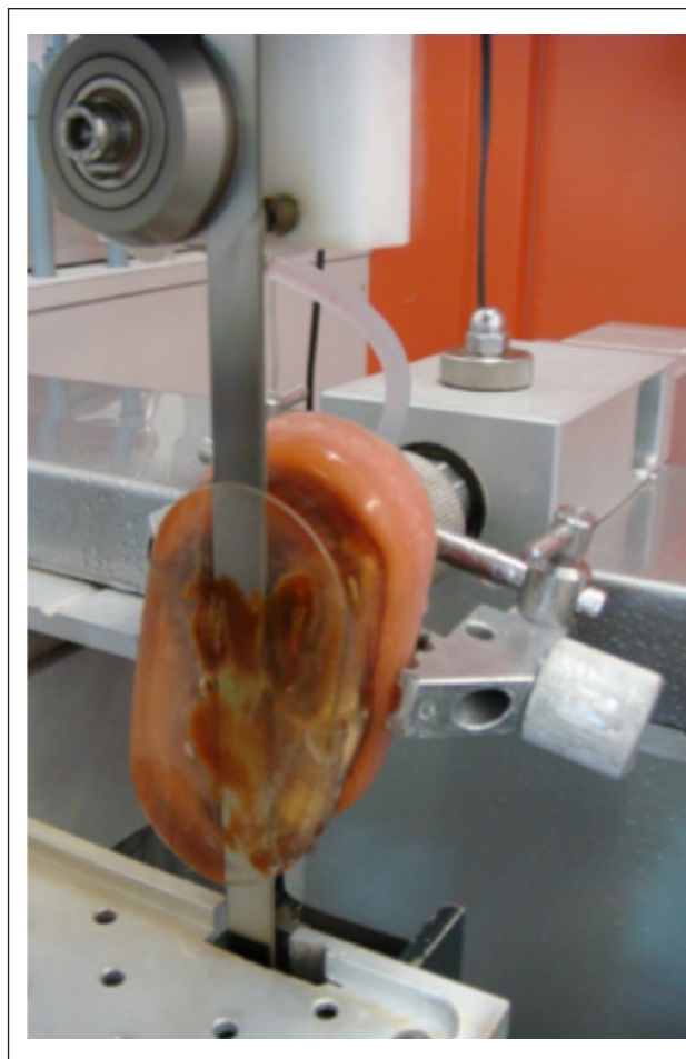
Figure 4 Whole feline stifle joint embedded in a methyl methacrylate block and undergoing sagittal slicing with a diamond-coated saw
